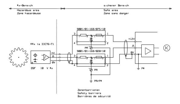
Connection diagrams (refer to dimensional drawing for exact type):
